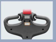
The upright-tiller running function allows it to work within confined space, such as container
